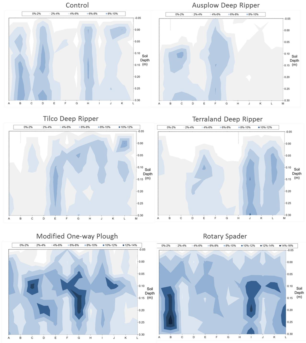
**Figure 2. Volumetric soil moisture (%) on soil pit faces treated with various strategic soil tillage methods for severely repellent pale deep sand at Irwin following 50mm of rain over 4 days. Pits were 140cm wide and 30cm deep. Darker shading is indicative of higher soil moisture content.**
