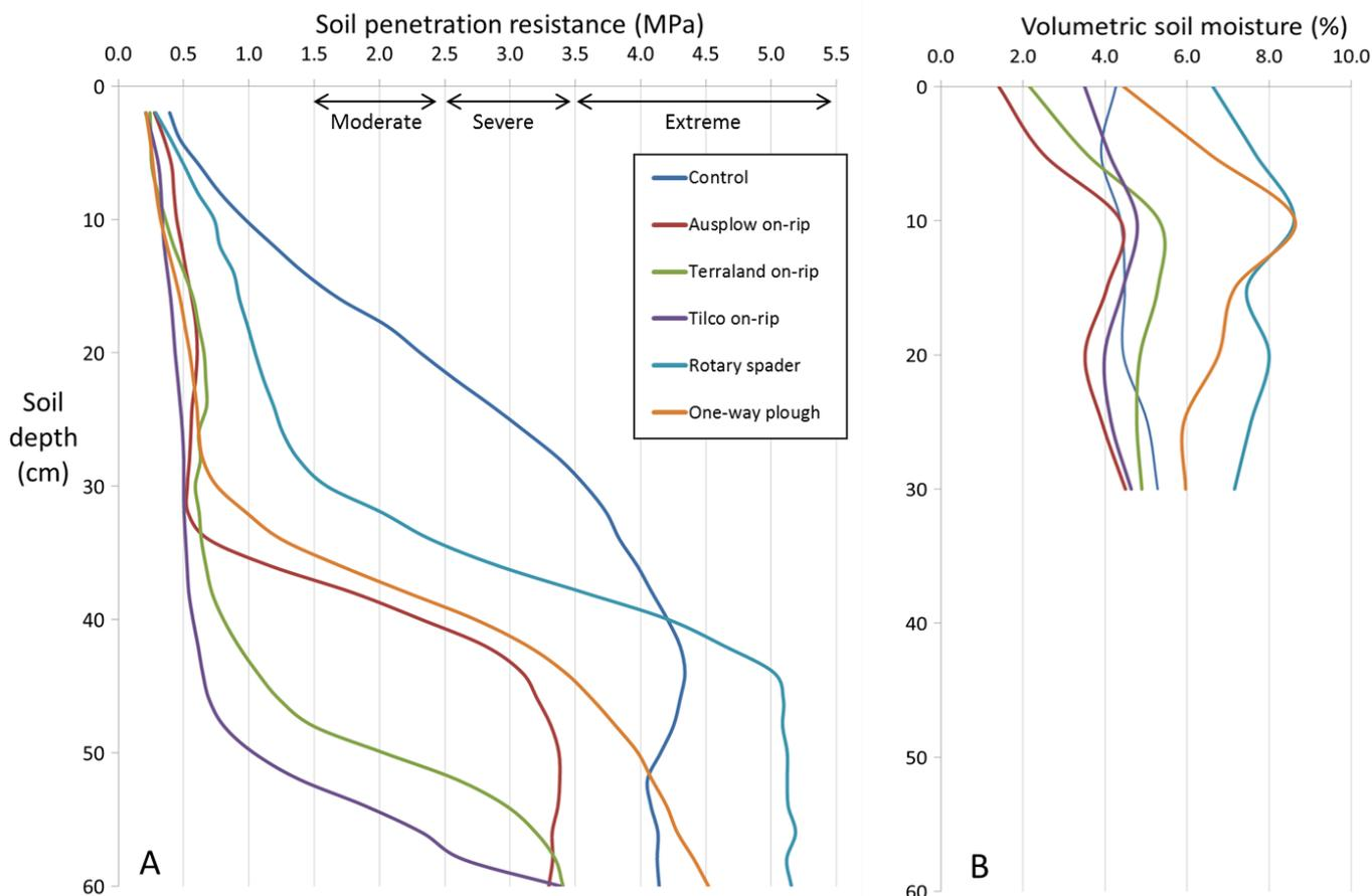
**Figure 1. A) Soil penetration resistance measured 31<sup>st</sup> May, and B) average volumetric soil moisture measured 25<sup>th</sup> May, in response to soil amelioration treatments for severely repellent pale deep sand at Irwin, 2016.** Note: Soil strength ratings (A) based on published reductions in cereal root growth rate, with severe reducing root growth rate by up to 75% and extreme preventing root growth except in pre-existing soil biopores and fractures.
